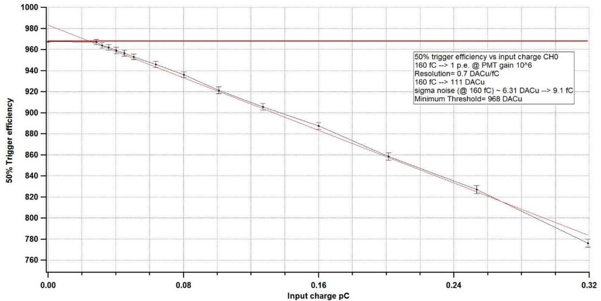
Figure 22. 50 % trigger efficiency versus injected charges.
