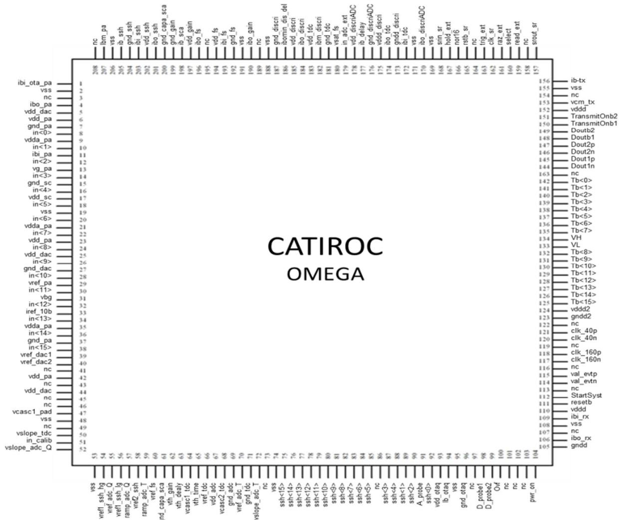
Figure 3 Pinout of CATIROC package
