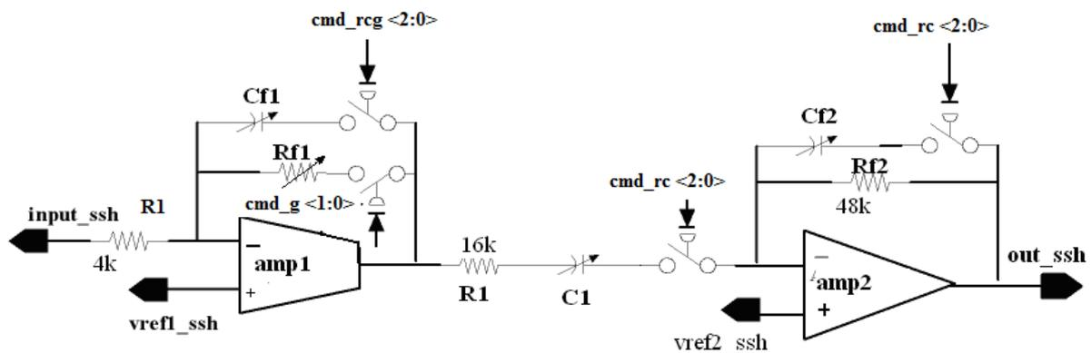
Figure 6 Slow Shaper schematic
