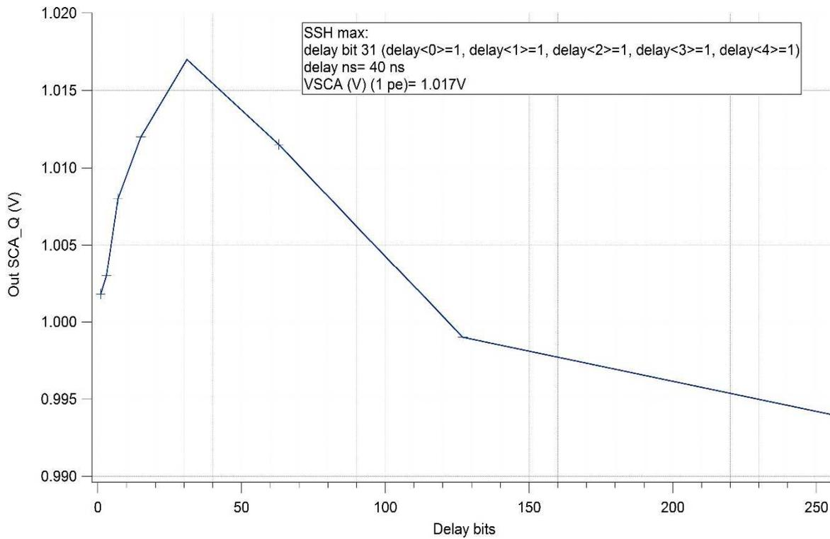
Figure 9 Value of the slow shaper hold signal vs delay. Optimum at delay= 31 (40 ns). Slow control bits: 221 to 228 in table3.
