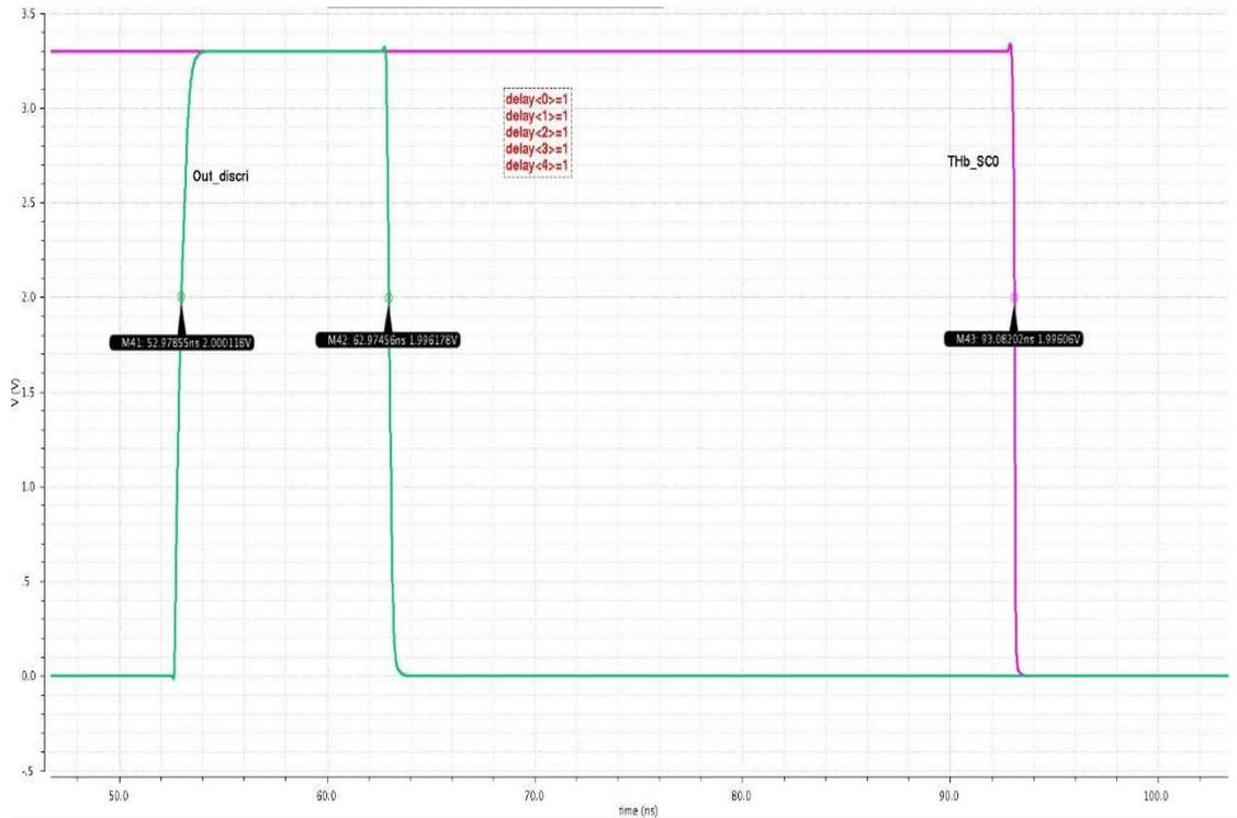
Figure 8 Output trigger and trigger delayed at the slow shaper maximum. (Slow shaper in default configuration).
