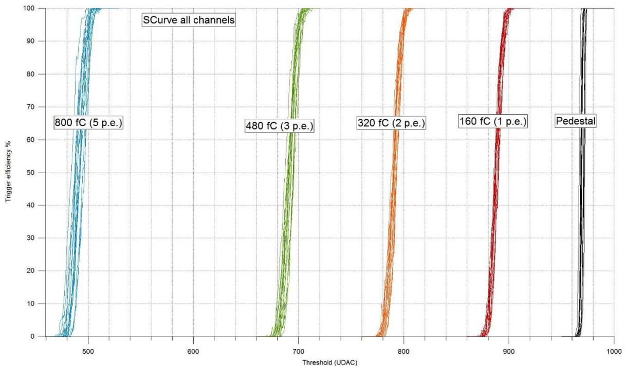
**Figure 21 Trigger efficiency vs threshold for various injected charges up to 800 fC (5 p.e.)**
