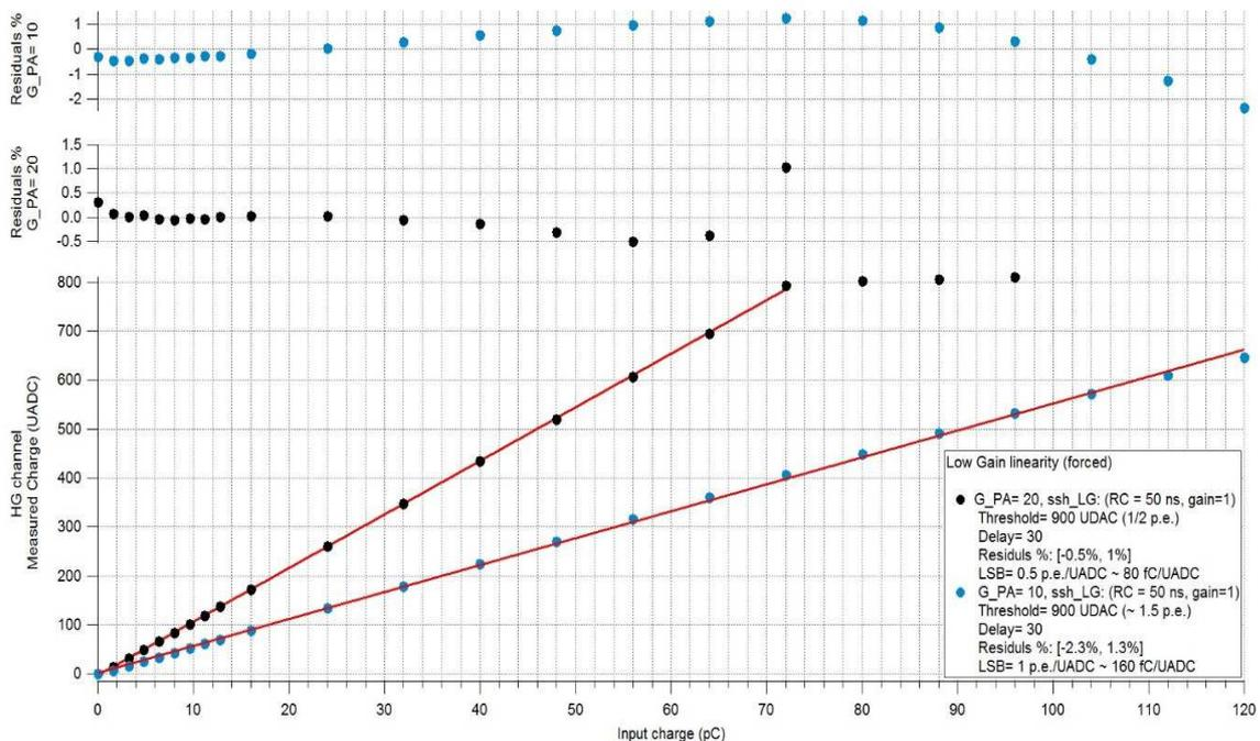
**Figure 31 Charge linearity channel 0, LG path for preamplifier gain 20 (black dots) and 10 (blue dots)**
