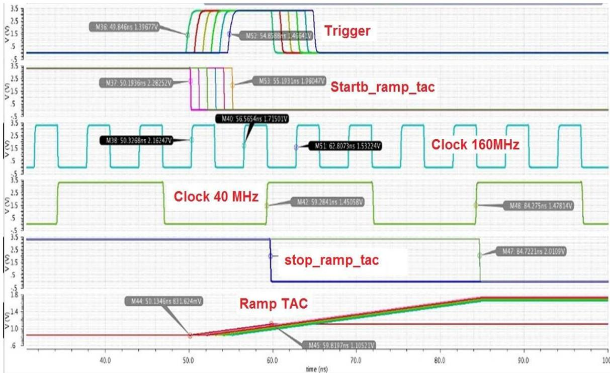
Figure 11 Trigger signal channel0 (at 1pe), Startb\_ramp\_TAC, Clock\_160 MHz, Clock\_40 MHz, Stopb\_ramp\_TAC, RAMP TAC.
