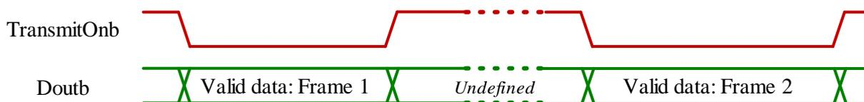
Figure 13 Chronogram of the readout frames
