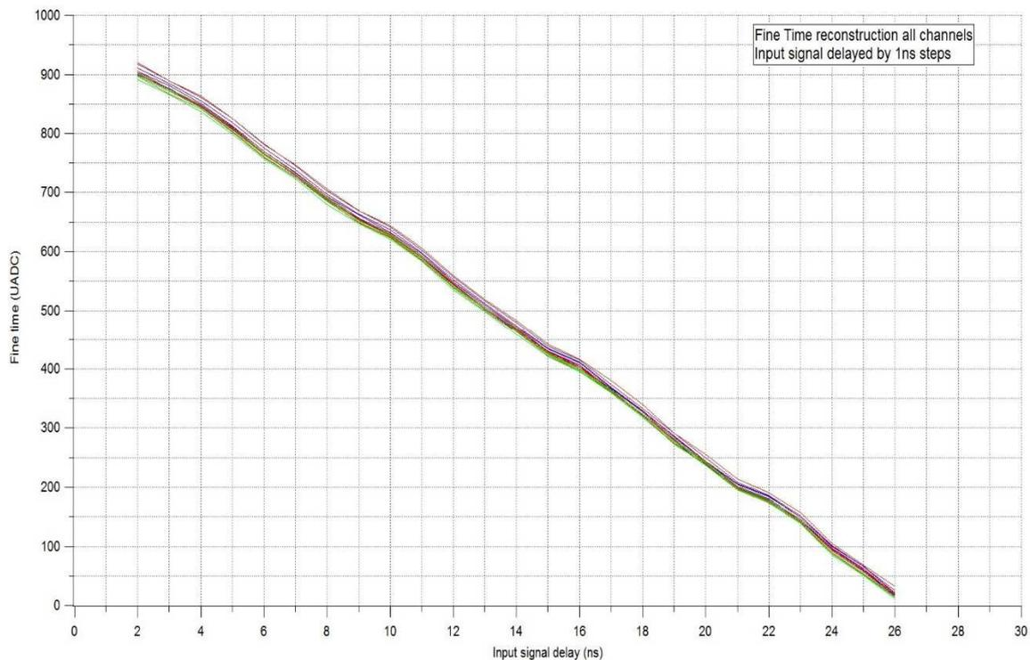
**Figure 36** TAC ramps for the 16 channels
