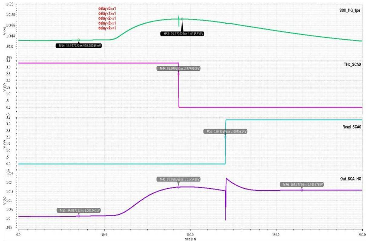
Figure 10 Shaper output signal for 1pe (SSH), trigger signal delayed to shaper maximum (Thb), Read\_SCA and SCA output signal (OUT\_SCA\_HG). Slow shaper in default configuration.
