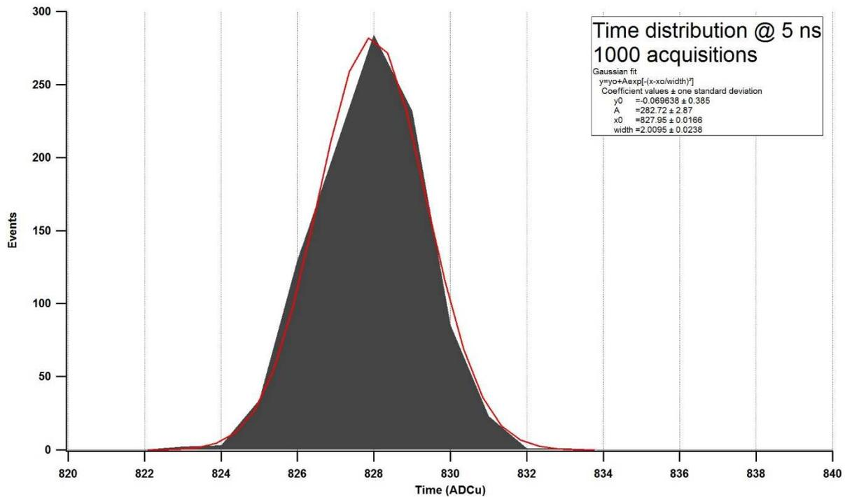
**Figure 35** Time distribution with an input signal delayed of 5 ns. 1000 acquisitions.
