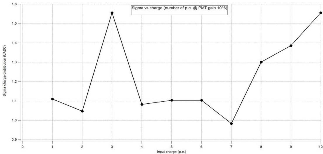
Figure 28 Sigma Gaussian fit of the charge distribution
