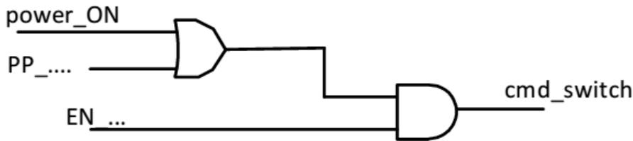
Figure 5 Power pulsing control logic
