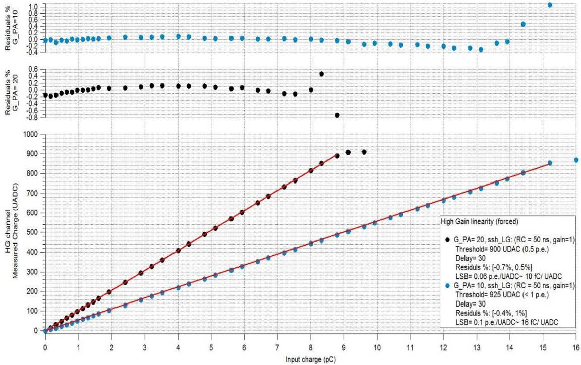
**Figure 30 Charge linearity channel 0, HG path for preamplifier gain 20 (black dots) and 10 (blue dots)**
