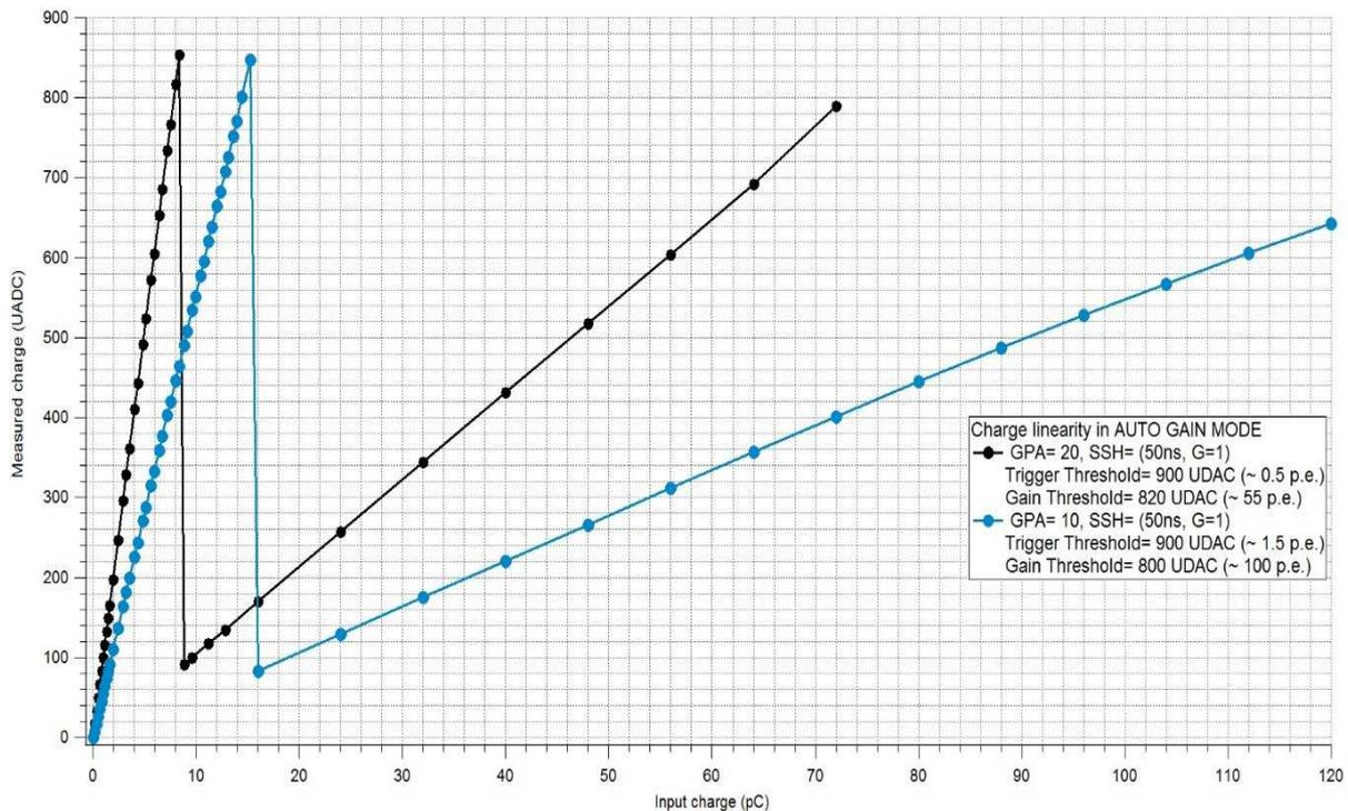
Figure 32 Charge linearity in Auto gain mode
