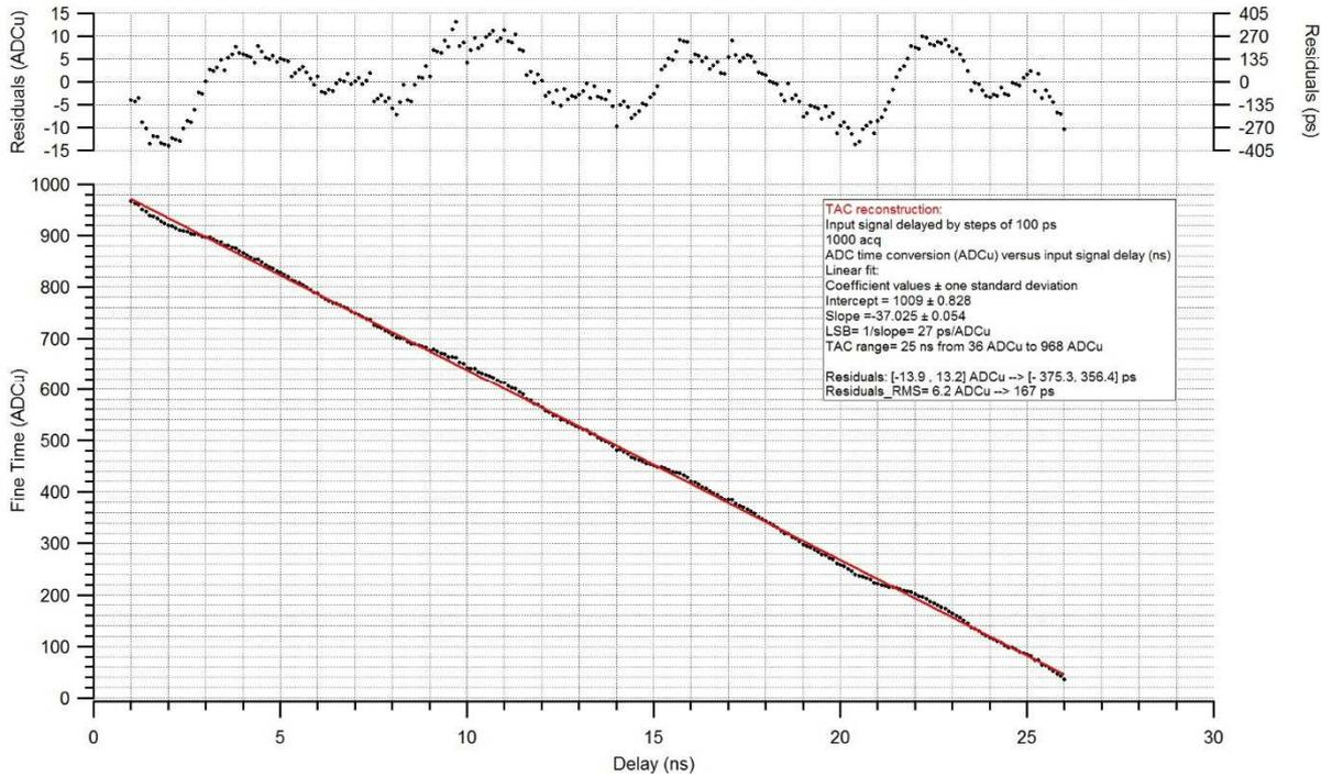
**Figure 33 TAC reconstruction with linear fit and TAC INL (ADCu)**
