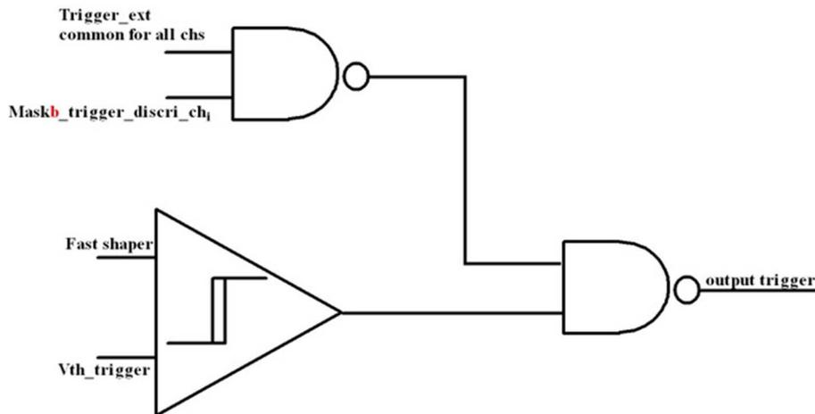
Figure 6 Mask and external trigger schematic
