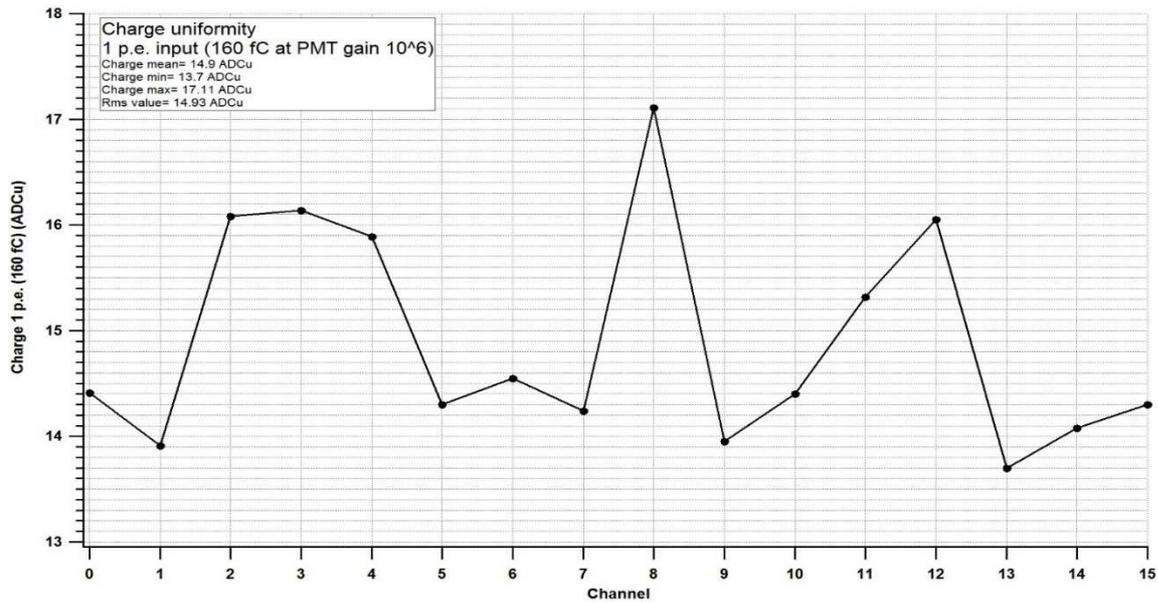
**Figure 29. Charge uniformity. 160 fC (1 p.e. @PMT gain 10<sup>6</sup>) injected in the 16 channels**
