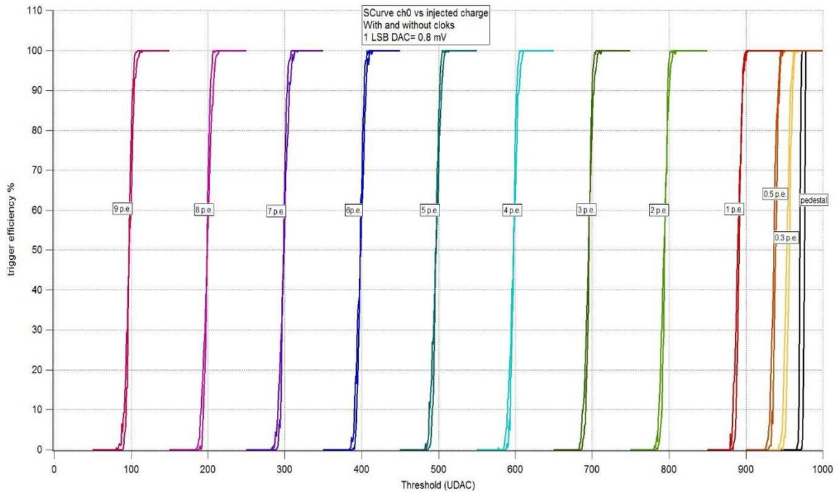
**Figure 20 Trigger efficiency vs threshold for various injected charges up to 1.4 pC**
