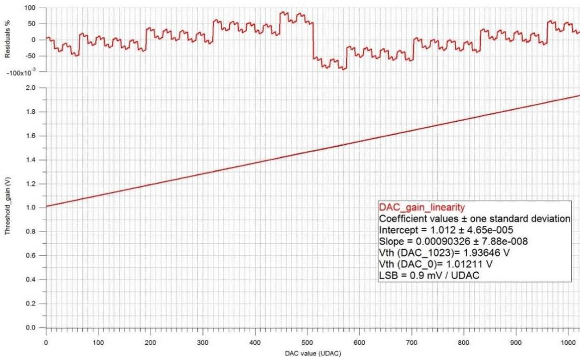
Figure 18 DAC gain linearity
