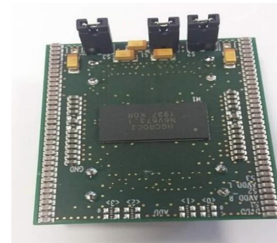
BGA on mezzanine
