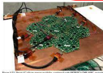
Figure 8.12: Seven 6" silicon sensor modules, equipped with SKIROC-CMS ASIC, mounted on a copper support (existing plane during the 2017 test campaign).
